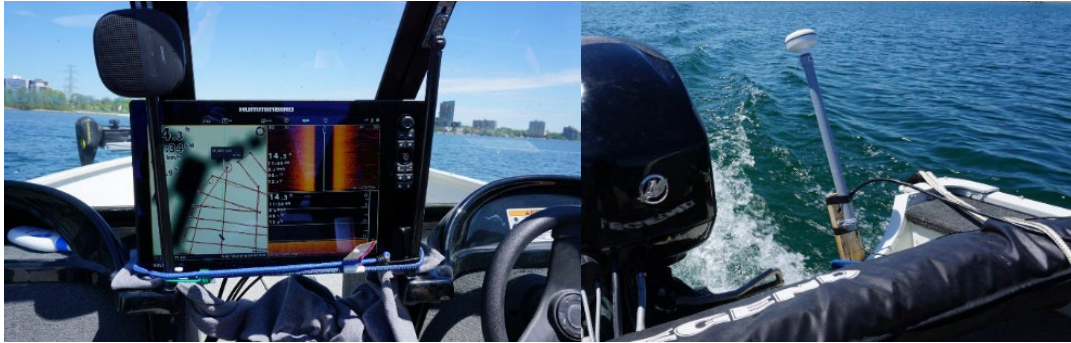
Figure 3.6 SOLIX data collection unit and transducer mount
