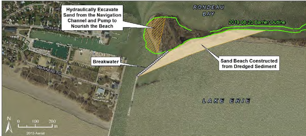
Figure 6.27 Part 1 Option 4-3 East Jetty Breakwater Extension and Nourishment
