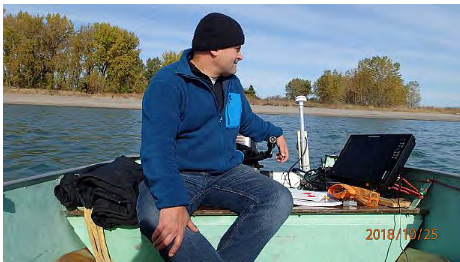
Figure 2.44 SOLIX Navigation Monitor (black, right) and GPS Antenna (back of boat)
