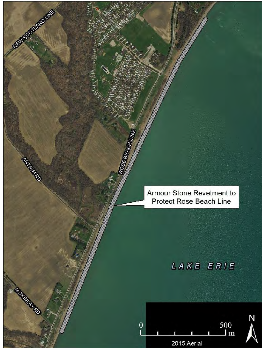
Figure 6.13 Rose Beach Line Armour Stone Revetment
